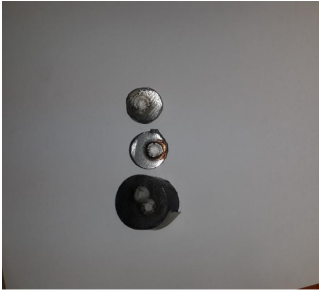
Fig 2.3: Sparked samples of Nissan Xterra, Toyota and Ford
